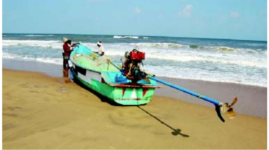
A traditional Andhra boat with an outboard motor fitted with long-tail propulsion unit
