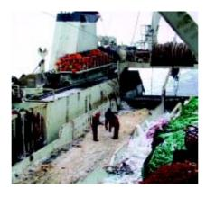
elevated surfaces, and open decks all pose significant hazards. OSHA regulations require that anyone exposed to a possible fall of 4 feet or more be protected, either by railings or by a fall arrest system.
