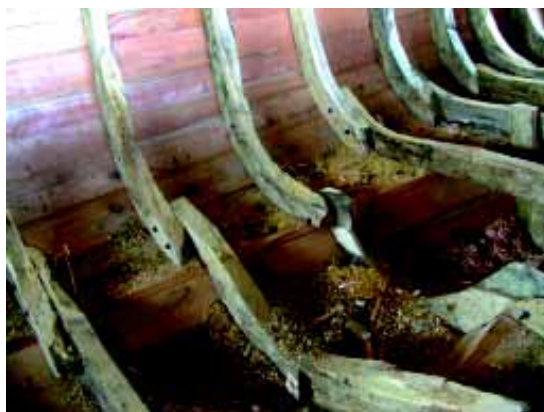
Examples of defective construction in post-tsunami boats from Aceh province, Indonesia.
