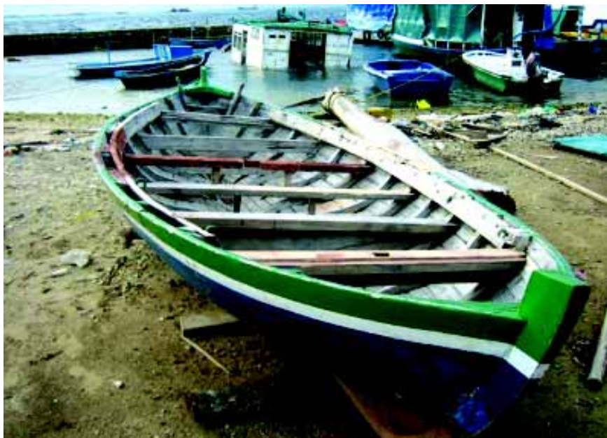
The Masdhoni of the Maldives. Some 50 Masdhonis, 85 ft long, are being built. Even 107 ft Masdhonis are under construction.
