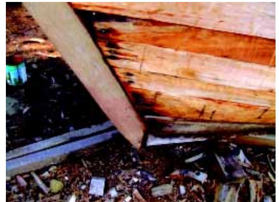
Examples of defective construction in post-tsunami boats from Aceh province, Indonesia.
