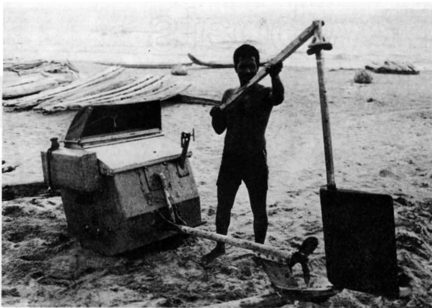
Above: The engine box with propeller shaft and rudder at Injambakkam near Madras. Below: This diagram illustrates a special feature of the retractable propeller and rudder, which “disappear” into a well in the hull when the craft reaches shallow water. Therefore no fixed keel is necessary.
