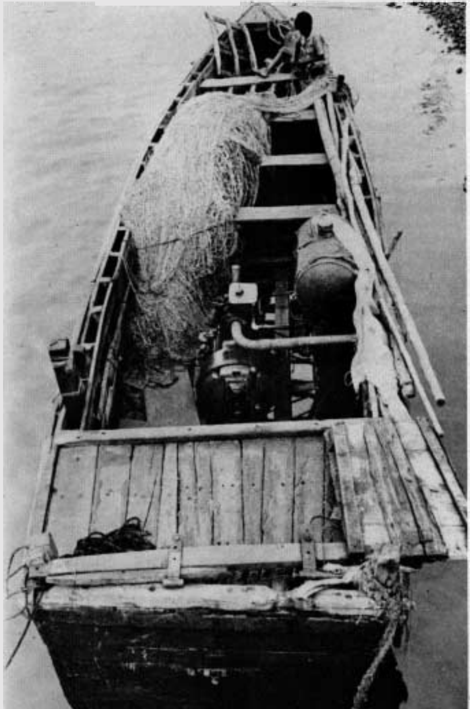
Motorized Nava with reversible gearbox and nets.
