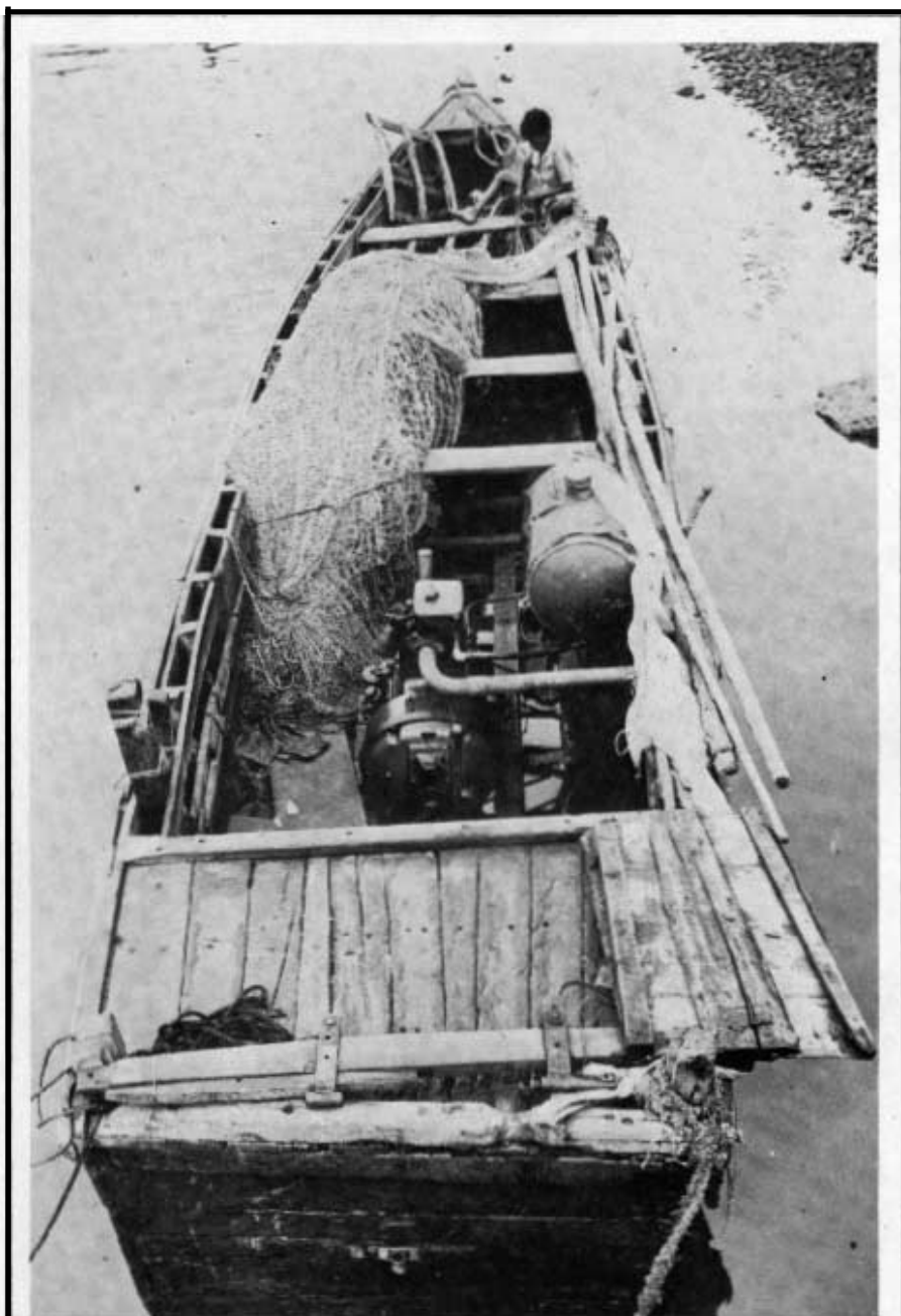
The motorized Nava of Kakinada. The motorization was carried out by the fisherfolk themselves on their own initiative.
