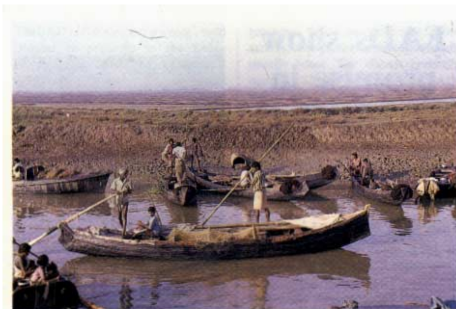
An 8m non-motorized nava near Kakinada, typical of those used in many local fishing communities.
