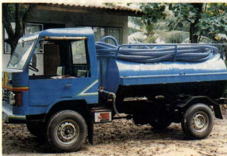
The 1000-litre mobile tanker with vacuum pump to drain oily bilge water from boats.
