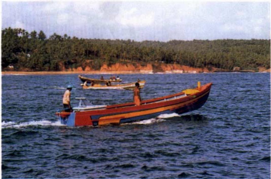
8.5 m plywood canoe, IND-28A, fitted with side mounted VST water-cooled diesel engine BOB Drive
