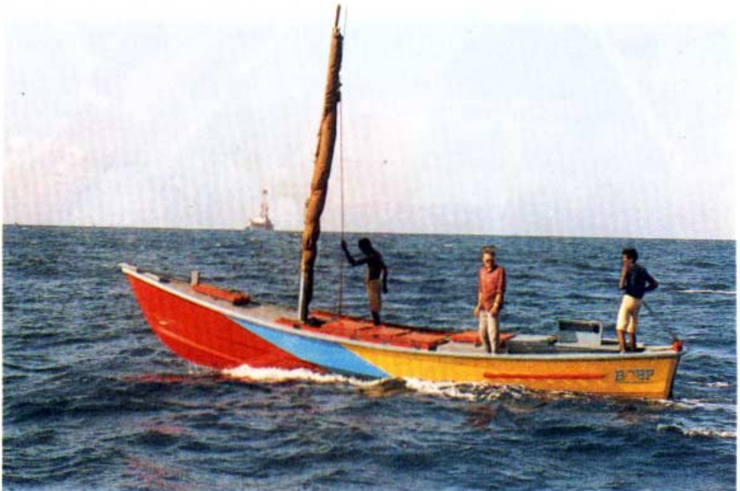
8.5 m FRP beachlanding craft, IND-20, fitted with side mounted VST water-cooled diesel engine BOB Drive
