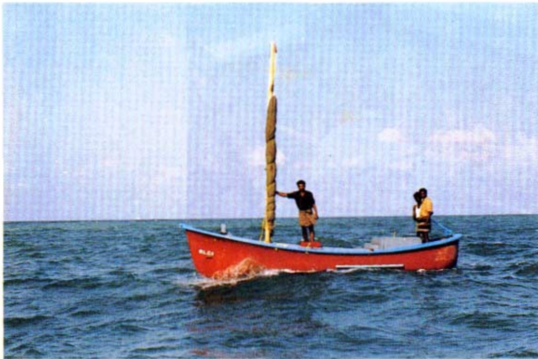
6.7 m FRP beachlanding craft, IND-25, fitted with top mounted VST air-cooled diesel engine BOB Drive
