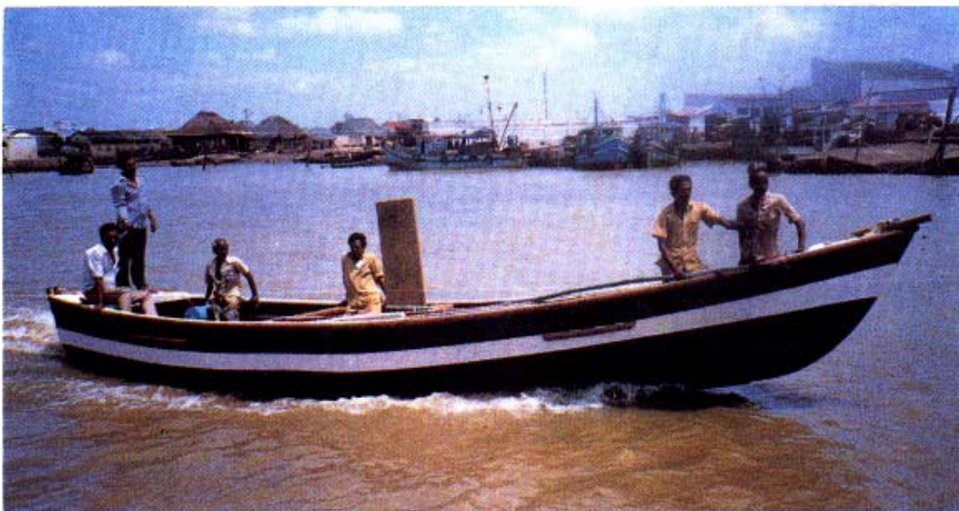
9.1 m FRP beach nava fitted with forward mounted Lombardini air-cooled diesel engine BOB Drive
