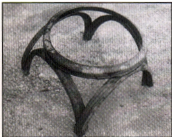
The stand of a local tyre garbage bin made from used truck tyres
