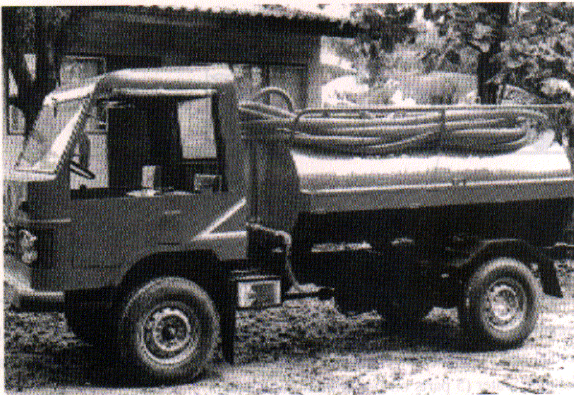
Figure 35b THE 1 m 3 MOBILE RECEPTOR FOR BILGE WATER AT PHUKET, THAILAND
