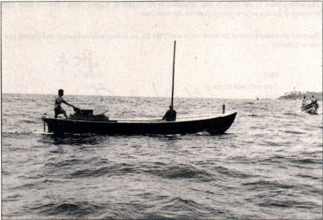
The IND-28, 9.1m with 9hp diesel water—cooled engine
