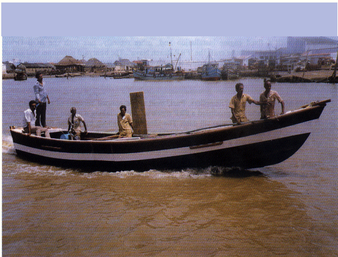
A FRP Beach Nava built by the APFC boatyard with the BOB Drive
