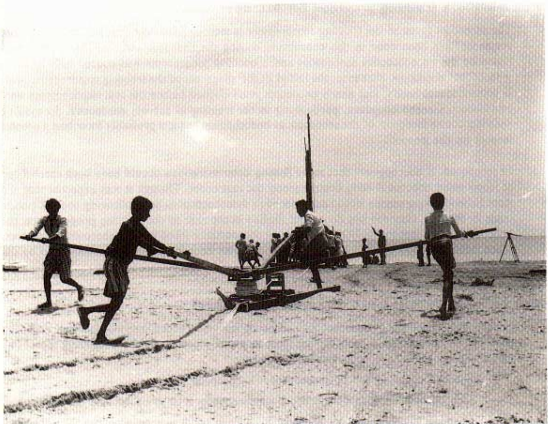
Hauling a BLC on to the shore with a steel winch
