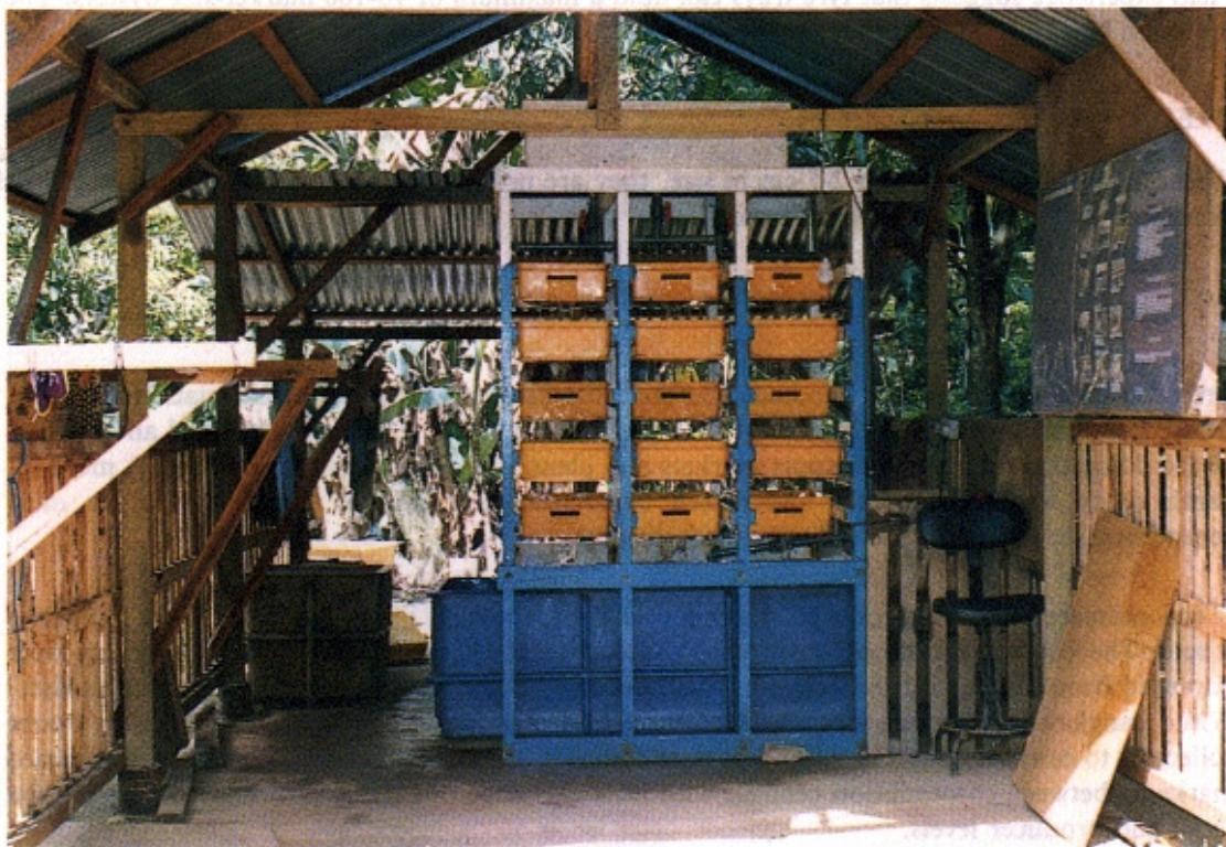
Small-scale depuration unit used by farmers.
