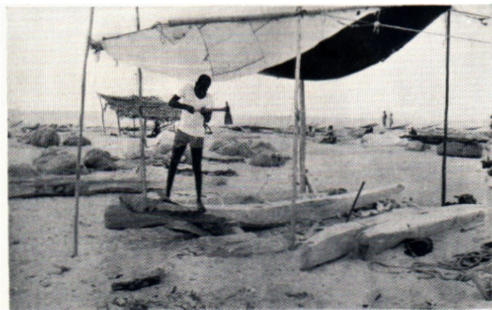
Logs are being carefully shaped and finished for a new kattumaram.
