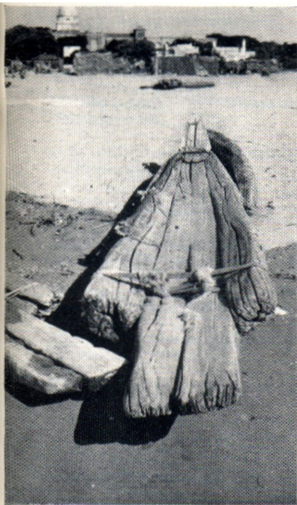
A set of assembled kattumaram logs that have seen many years of rough use.
