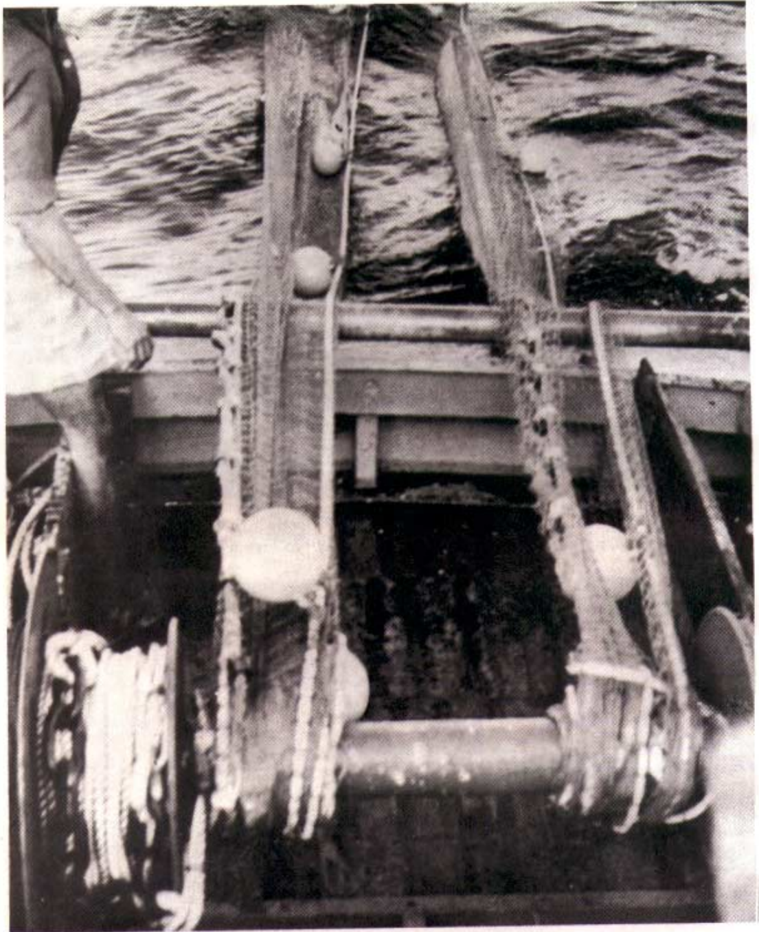
Net being hauled through a net-drum mounted on the deck.
