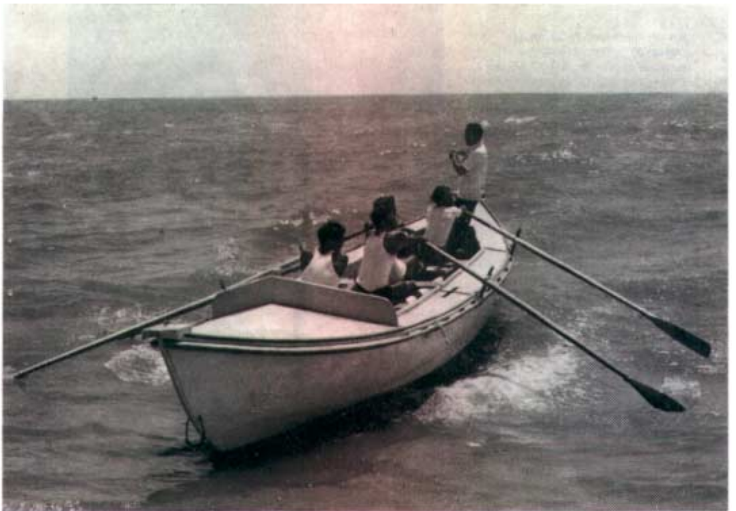
The BOBP-designed craft IND-17 under sail (Figure 1, right) and on a rowing trip (Figure 2, below). The craft weighs only slightly more than a canoe, but its volume is considerably more than a canoe's.
