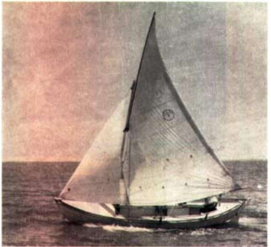
The BOBP-designed craft IND-17 under sail (Figure 1, right) and on a rowing trip (Figure 2, below). The craft weighs only slightly more than a canoe, but its volume is considerably more than a canoe's.
