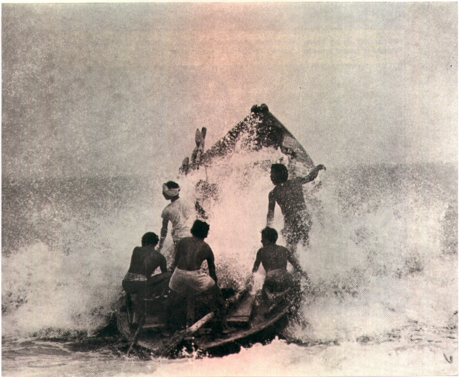
Right: IND-13 crew prepare to launch the boat. Below: The boat crosses the surf. The boat performed much better than the traditional nava during commercial fishing trials using the same amount of fishing gear.
