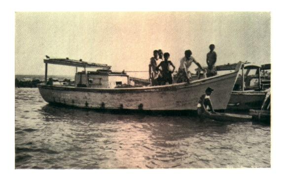
The photographs shown here were used for the fishing gear improvement project. Top: The 28-feet-lon9 3½-tonnermade of fibreglass reinforced plastic and fitted with a 33—H.P. engine, that was used in Beruwela.
