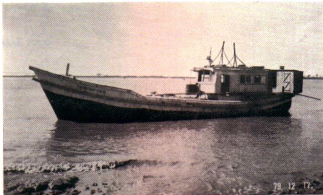
Miriam 9 (top) and Miriam 18, both fishing boats belonging to the Kalidaha fishing project, were used for the experiments to improve the large-mesh driftnets. Miriam 9 is a 12-m wooden boat driven by a 22-H.P. engine; Miriam 18 is a 13 m ferro-cement boat with a 33 H.P. engine.
