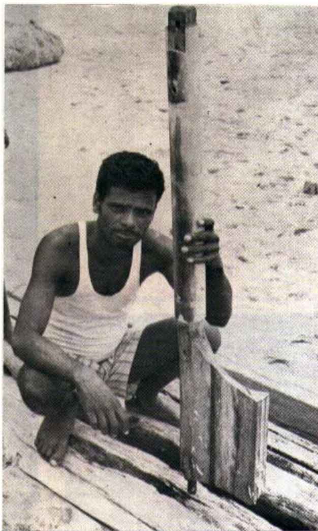
Fish tail rudder with PVC lined stock.
