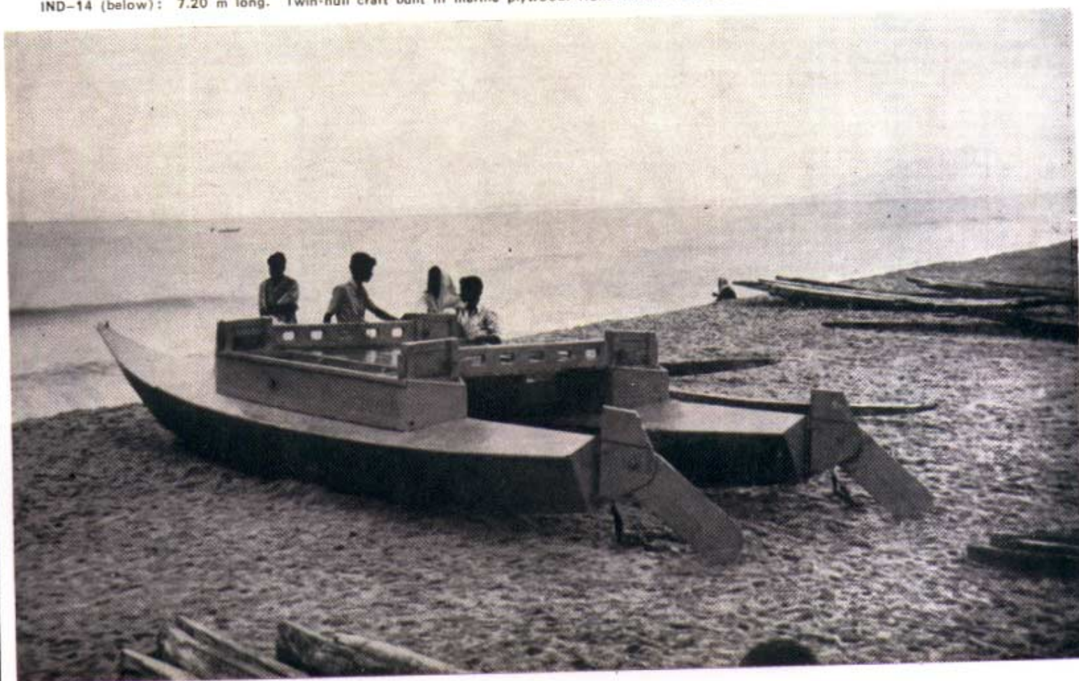
IND-14 (below): 7.20 m long. Twin-hull craft built in marine plywood. Hulls decked forward and aft.
