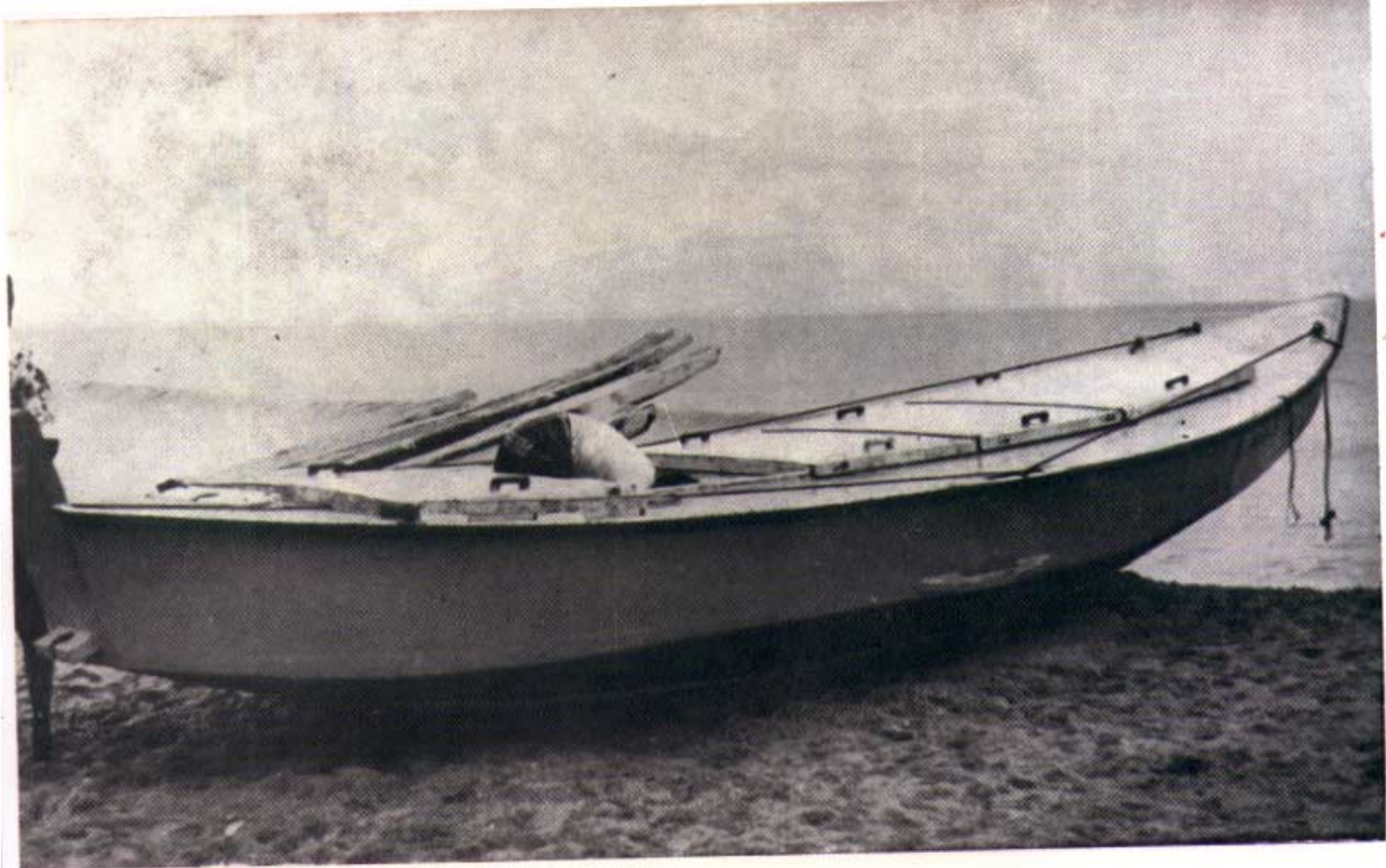
IND-13 (above): 7.40 m long. Decked, built of marine plywood. Equipped with sail and 5 hp inboard engine. One of the two prototypes selected for intensive fishing trials.
