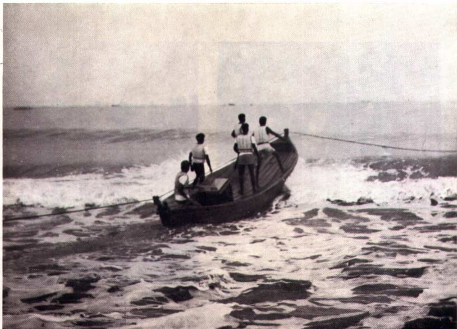
IND-11 using the rope system to cross the surf. Note fore and aft rope fairleads with locking arrangement.
