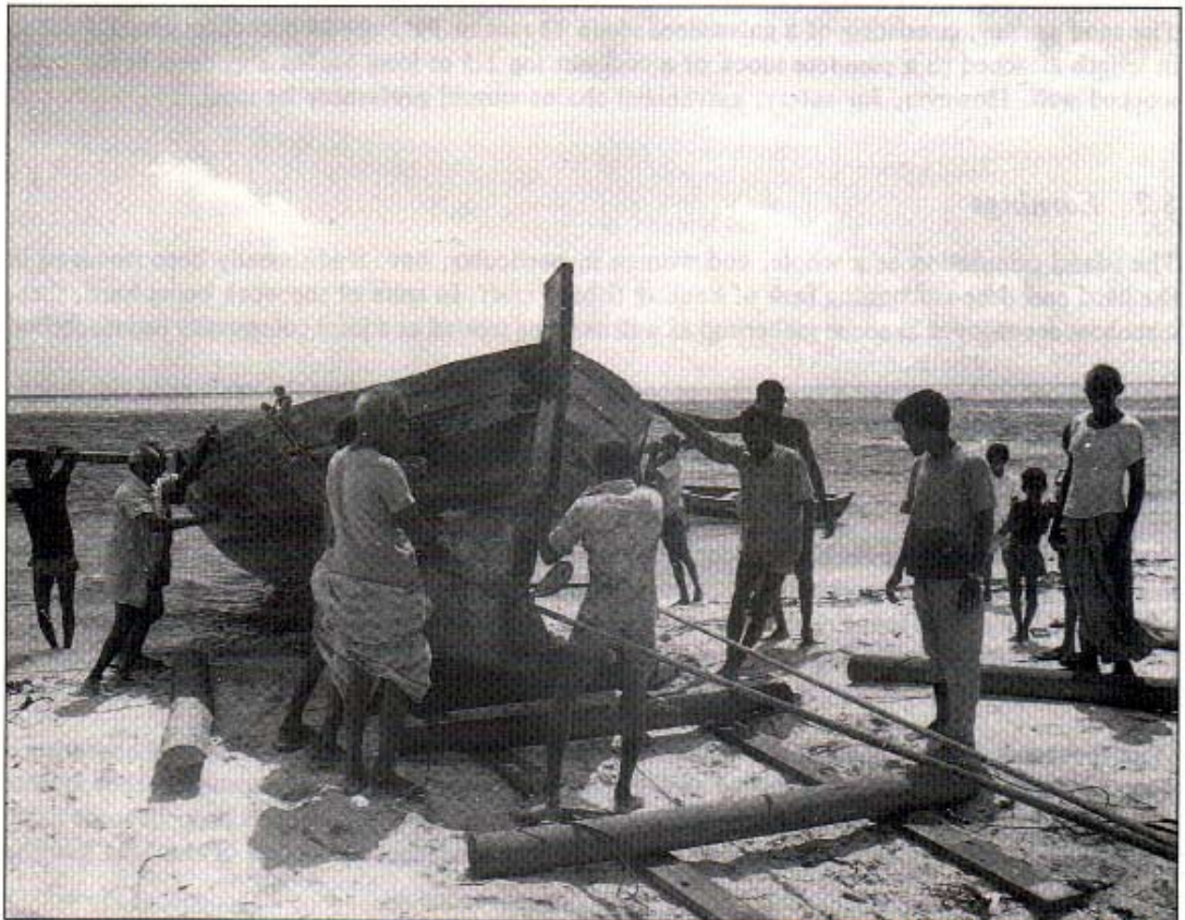
The dhoniis hauled on to the rails and rollers
