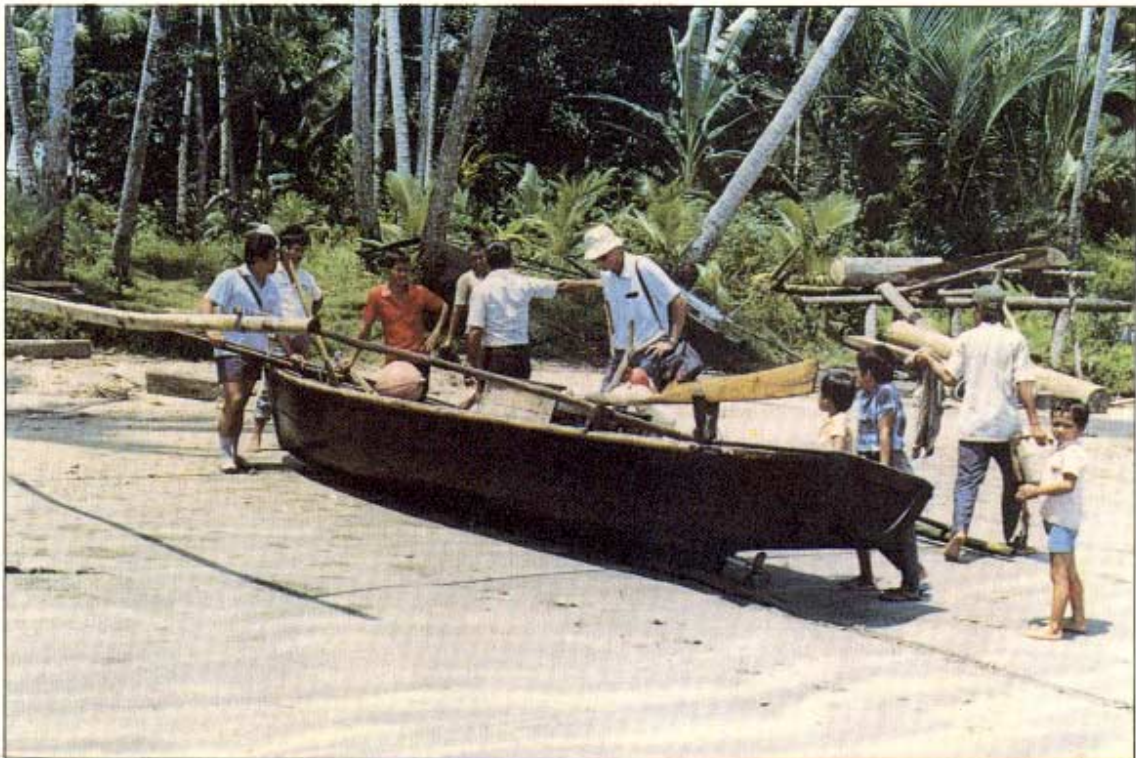
Inboard motorized dugout outrigger canoe (5-7 m)
