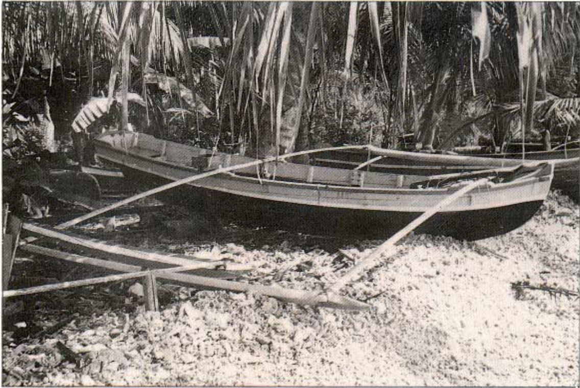
Outboard motorized dugout outrigger canoe (5-7 m)
