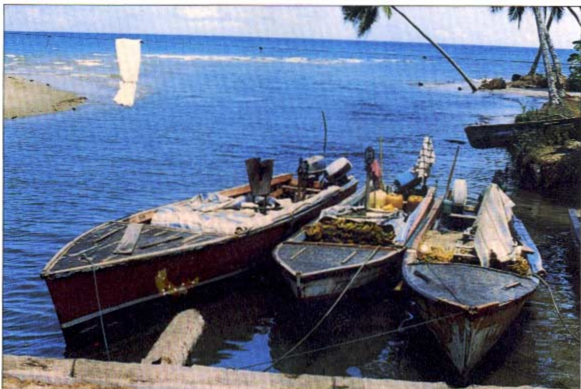
Outboard motorized plankie open boat (1-10 m)
