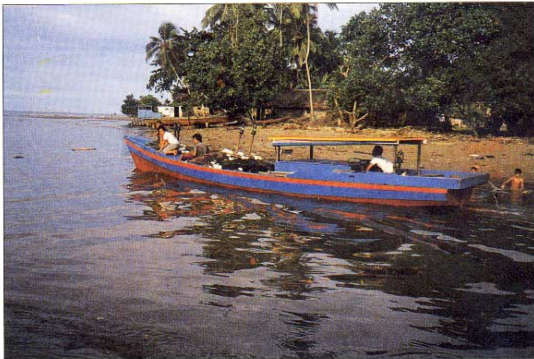
A larger inboard motorized half-deck drifnetter (10-12 m)
