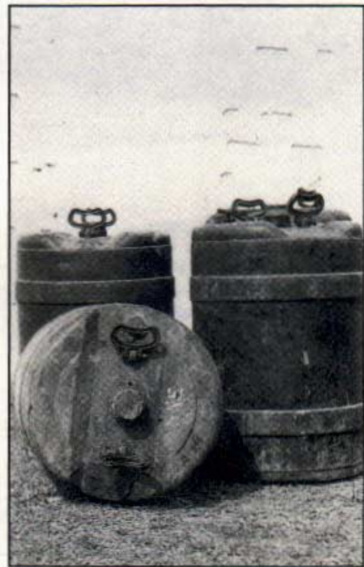
100 l plastic drums used as floats for the cage
