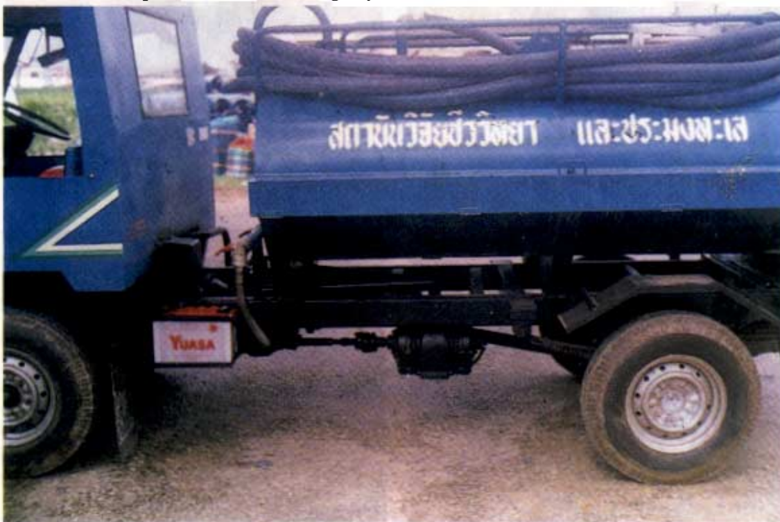
Phuket harbour's oily waste reception truck. Note pump driven from 'power take-off unit'.
